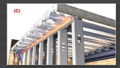
For fluted deck, install header track to fluted deck as recommended by manufacturer. Friction fit Track-Safe™ to header track on one side of wall before or after stud installation, no mechanical fastening required. (C) On one side of wall assembly spray approved RectorSeal sealant over mineral wool and track safe as required by UL system. (D) Install wall sheathing over Track-Safe™ to complete wall assembly.
