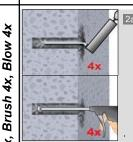
2a. In case of standing water in the drilled bore hole, all the water has to be removed from the hole (e.g. vacuum, compressed air, etc.) prior to cleaning.
