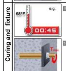
Allow the adhesive anchor to cure to the specified full curing time prior to applying any load (see Table 3).
