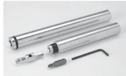
The 516 tool (ELP400) is a two step installation tool for use with all drive styles and lengths of 5/16" Ultracon fasteners. The standard 6" sleeve will install fasteners up to 4" long. For 5" and 6" long Ultracon fasteners, an 8" sleeve is required.
