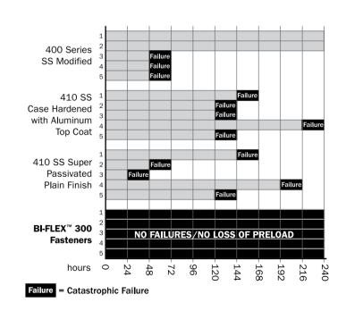
All fasteners were placed through a clear hole in 6061 T6 aluminum with a thickness of 0.125" and drilled into an unplated steel strip measuring a thickness of 0.125". A strip of 0.060" aluminum was placed in between the 0.125" aluminum and steel strip on one side, to simulate a fastener placed under load.
